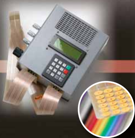
In 1999, the researchers built a “tongue display unit” with a stimulation system (inset) that would sit on the tongue.
